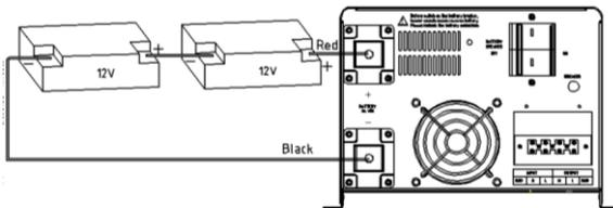
(Note that the red cable is connected to the positive terminal, black cable is connected to the negative terminal, and 2500W battery cable is more than 35mm<sup>2</sup>, 3500W battery cable is more than 50 mm<sup>2</sup>)
